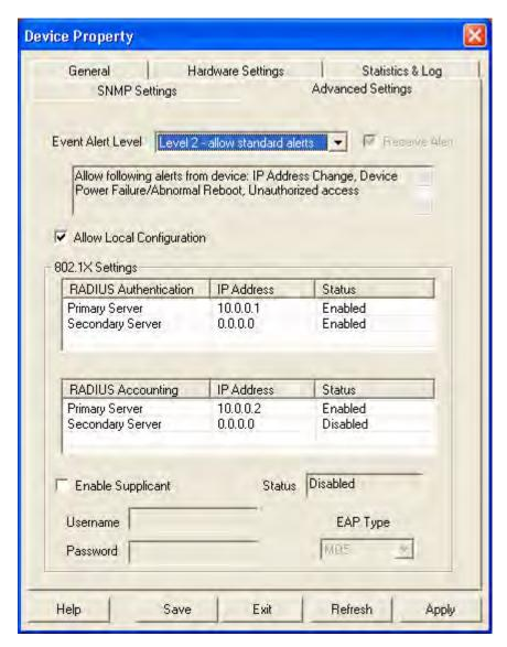
17 You can view the Event Alert Level and 802.1X Settings configured for this particular NJ220. 802.1X is a security protocol for LANs that relies on the Extensible Authentication Protocol (EAP) to pass messages to RADIUS authentication servers.
